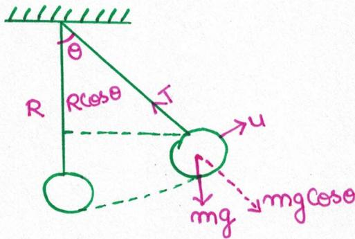
$$T - Mg \cos \theta = \frac{Mv^2}{R} \quad (\text{equation of circular motion}) \quad \text{--- (1)}$$
