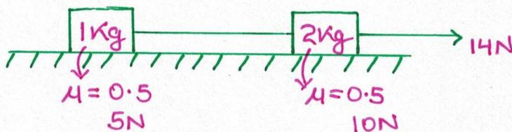
We start adjusting friction from 2 kg block
